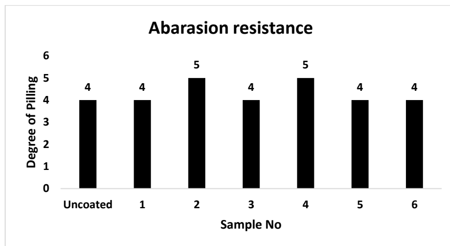
Figure 10. Degree of Pilling of screen-printed samples
