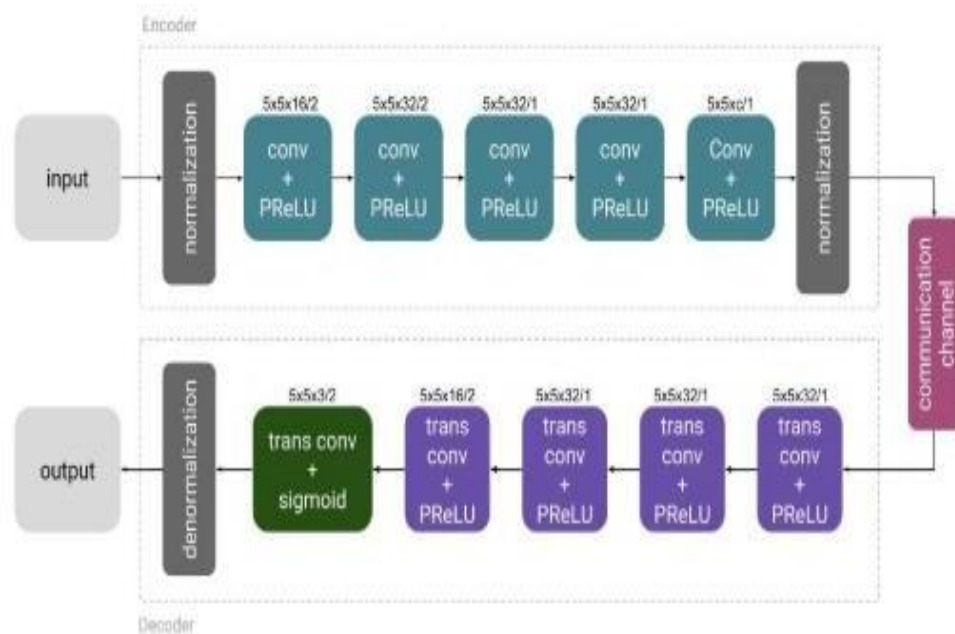
Fig.7. The architecture of the encoder and decoder for the CNN scheme
